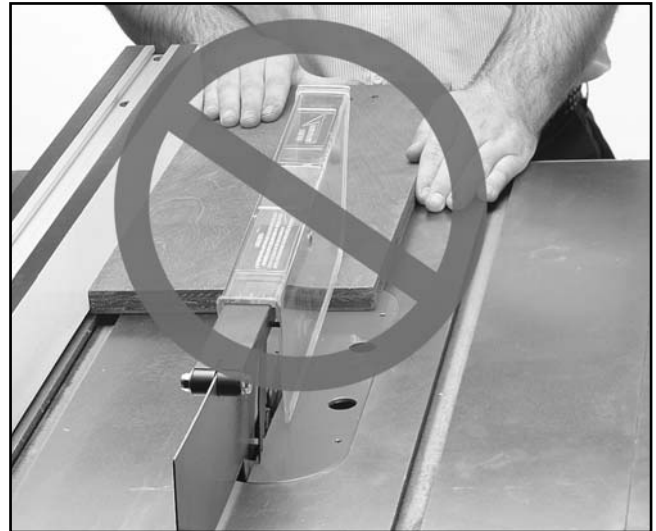
Figure 37. Do not stand directly behind wood.
